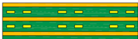
Two differential pairs per routing channel (Only 2 high speed signal layers required to route 6 differential pairs)
