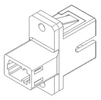
This optical adapter enables direct optical connection between an SC plug and an LC plug despite their different ferrule diameters (SC plug: Dia. 2.5, LC plug: Dia. 1.25). Low insertion loss and high durability are ensured by using a precise zirconia ceramic split sleeve insert. In addition, this adapter can be applied to the same panel pattern as a normal SC adapter without any modification.
