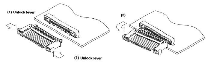
The plug should be pulled out with 15 ° (Max.) diagonally to the width direction.
