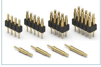
Mill-Max has added three new heights to the popular 0914 series of spring-loaded pins and corresponding single and double row connectors. The 0914 series has a mid-stroke distance of .045" (1,14 mm) [.090" (2,29 mm) full stroke] – close to double most standard series products. This provides more flexibility and tolerance for your assembly. These new, taller versions can be useful for assemblies requiring greater distance between mating surfaces and contact points.
