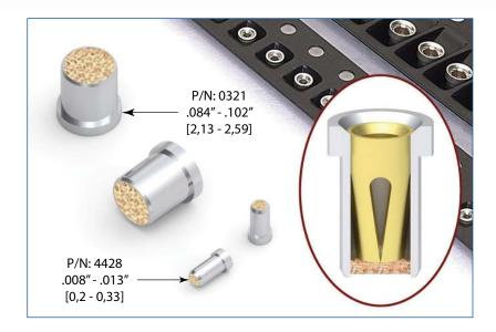
Mill-Max has added a micro-miniature option to our organic fibre plug<sup>®</sup> receptacle lineup. The newest Mill-Max socket receptacle, 4428-0-43-15-04-14-10-0, is our tiniest OFP<sup>®</sup> receptacle ever. Optimized for high-density packaging down to 1 mm pitch, this micro-miniature, ultra-low profile receptacle accepts .008"-.013" device leads or mating pins and can be soldered into a hole as small as .030."
