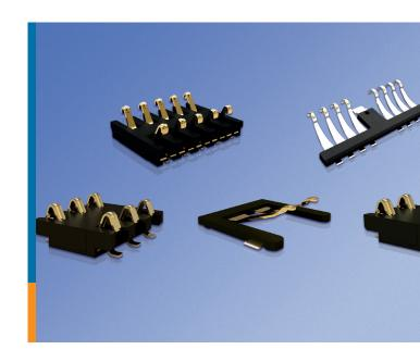
TE Connectivity introduces new compressive board to board connectors. These are low cost, highly reliable and versatile connectors, used to provide either power or signal connections between either two printed circuit boards or one printed circuit board and another electrical module. This product series helps save cost and space in most consumer electronic devices.
